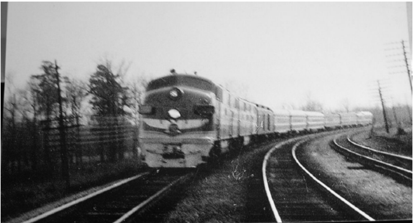
Taken in the early 1950's, the MoPac was re-painting all passenger equipment to the Eagle paint scheme. Heavyweight coaches were being "modernized" with large picture windows and skirts added. Following the two E7 units on this train No. 220 coming around the curve formally called County Hospital, now a new Westinghouse plant occupies the grounds, is a 4100 Baggage/Express car, two (2) 6300 modernized coaches, one (1) 870 lightweight Grill/Lounge/Coach, one (1) 8-5 Clover Heavyweight-Standard sleeping car, one (1) 10-6 Eagle lightweight sleeper, and bringing up the rear is Parlor-Observation Car #10603, which in a few short years will be pulled out of service and rebuilt into Business Car No. 8 and named THE EAGLE. This picture made in late March is somewhat grainy, as sleet is just beginning to fall. The extra sleeping car is in route from Hot Springs to Chicago and reflects the increased patronage during the Oaklawn Park Race Track season. ( John A. Mills photo )
