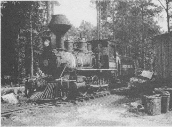
Reader RR Engine #4, a 2-6-2- built in 1913, an oil burning engine weighing 68 tons. Seen in 1985, (Ken Ziegenbein photo)
