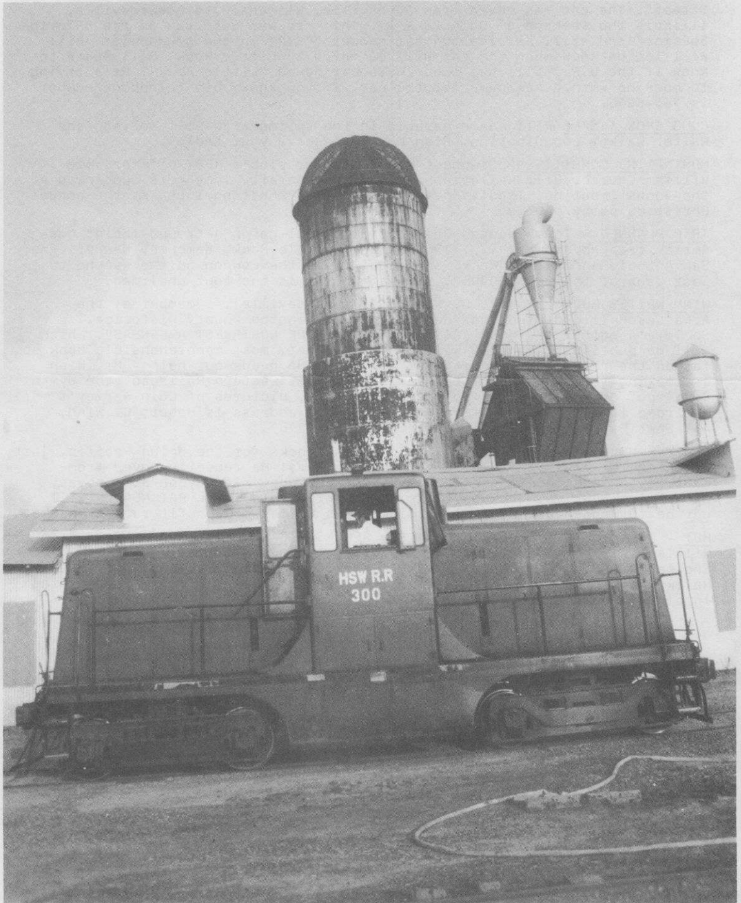
Helena Southwestern Railroad Company's #300 (a G.E. 45-ton locomotive bought new in 1948) goes to work on a sunny, hot July 18, 1986 in West Helena, Arkansas. She was hosed down just before this photo was made. (Ken Ziegenbein, photo)
