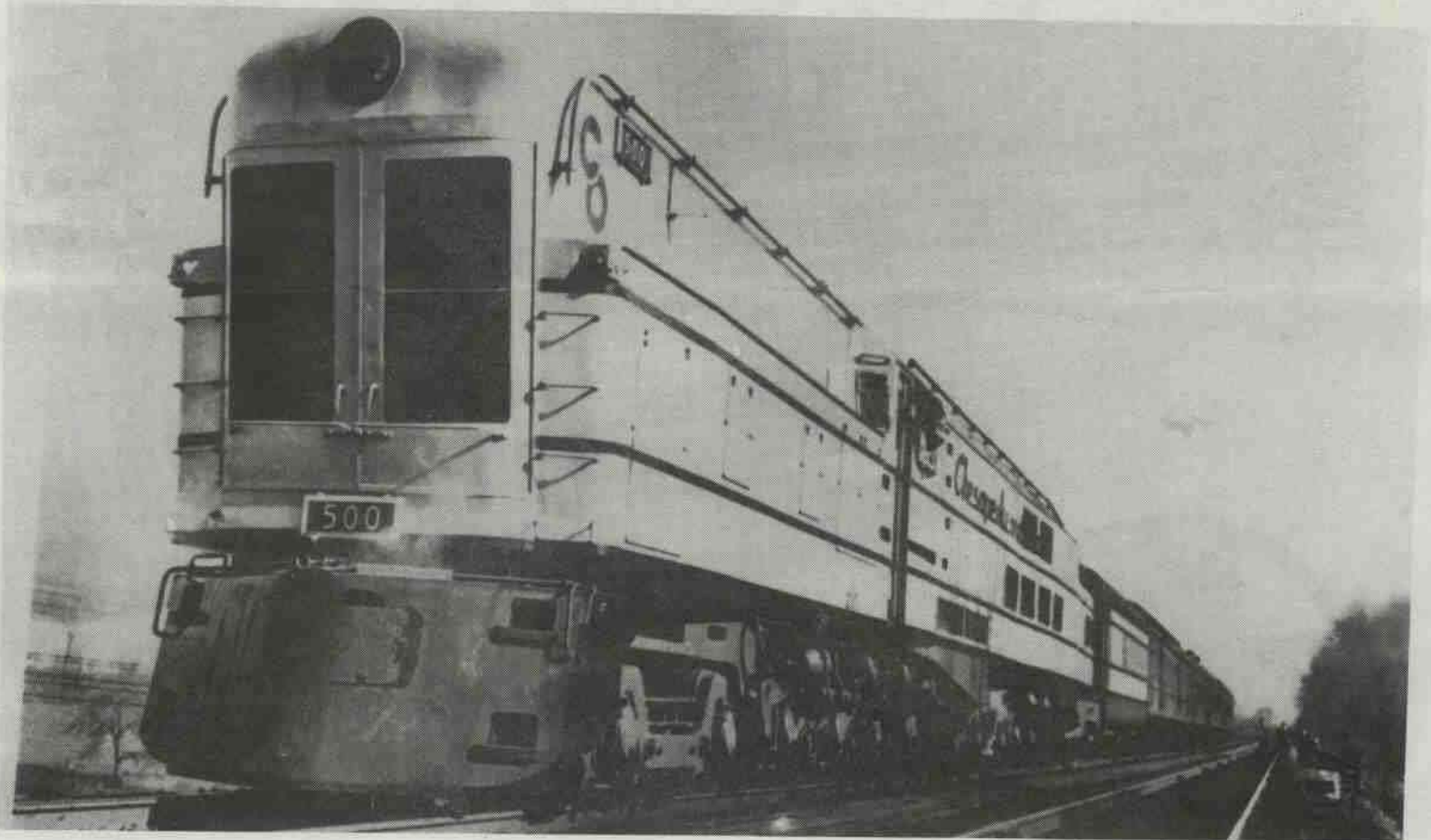
Shown near Cincinnati, Ohio in 1948 is Chesapeake & Ohio No. 500, the world's first steam turbine electric locomotive. Coal compartment is in the front section. A stoker feeds coal to a firebox in the center section, where also is a 6,000 HP turbine, and 2 - 2,000 KW generators which supply current to 8 motors mounted on the axles. The last unit is a water tank. The engine was 154 feet long, the longest steam locomotive ever built. There were electric and air brakes. It was called "Sacred Cow." Built by Baldwin in 1947 with 98,000 lbs T.E., weight 1,233,970 lbs, boiler pressure 310 lbs., carried 29½ tons of coal and 25,000 gallons of water. Three such engines were built. (CLIFTON E. HULL collection)
