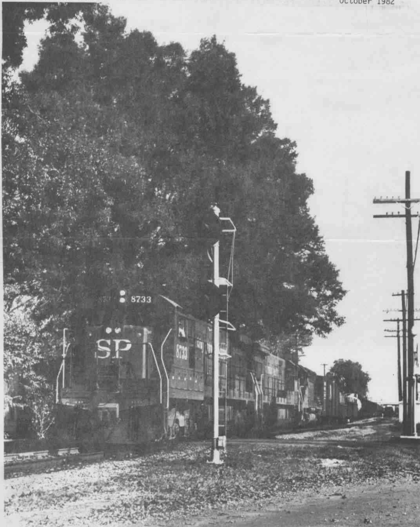
A SOUTHBOUND COTTON BELT manifest passes the last signal out of Pine Bluff Yards and onto the Main Line to Texarkana. The heavy power consists of G.E. U33C #8733 a sister U33C, and an EMD SD-45, a total of 10,200 horsepower, leading loads towards the great Southwest. Photo in the Fall of 1981 by John M. Martin
