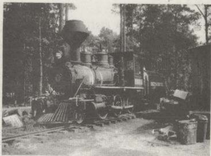
Engine #4, a 2-6-2 built in 1913, an oil burning engine weighing 68 tons.
