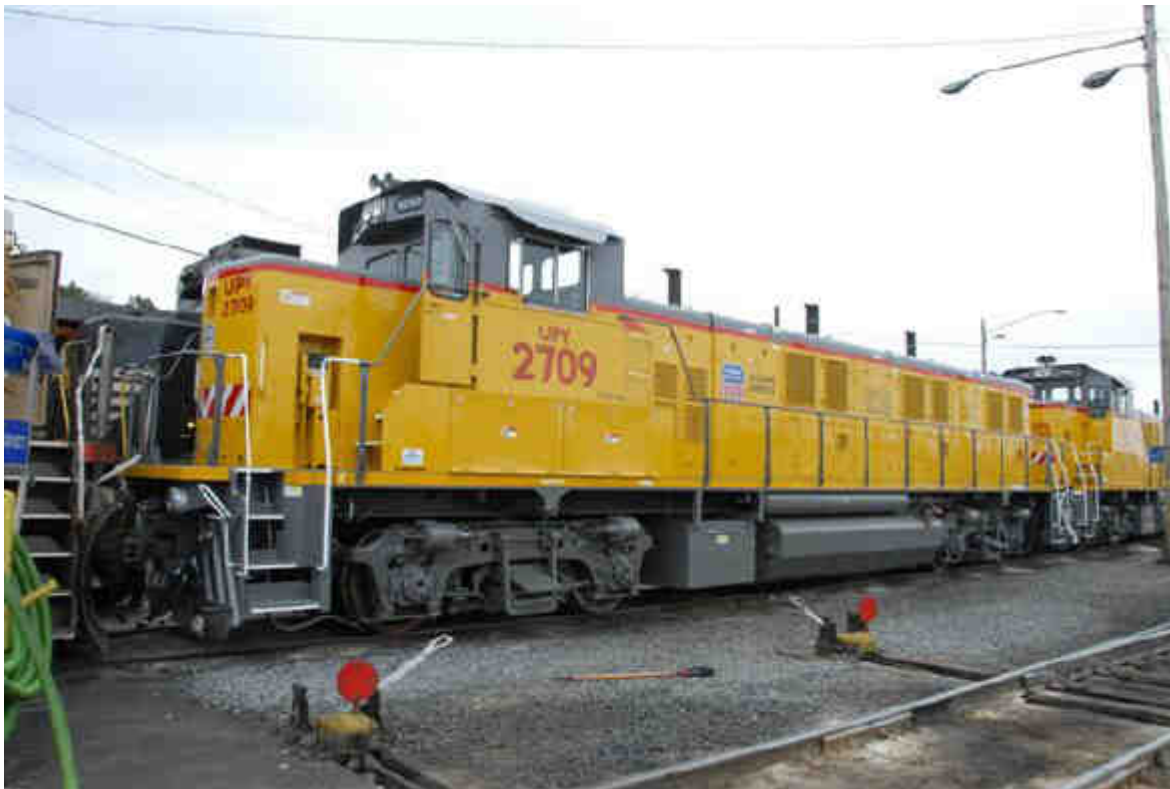
UPY 2709 in North Little Rock in February 2007. This is a new 2100 hp energy-efficient locomotive and they say it's very quiet. It is 74 feet long and holds 1,940 gallons of fuel. It was built by EMD and is classified as a GS-21B. (John C. Jones photo)
