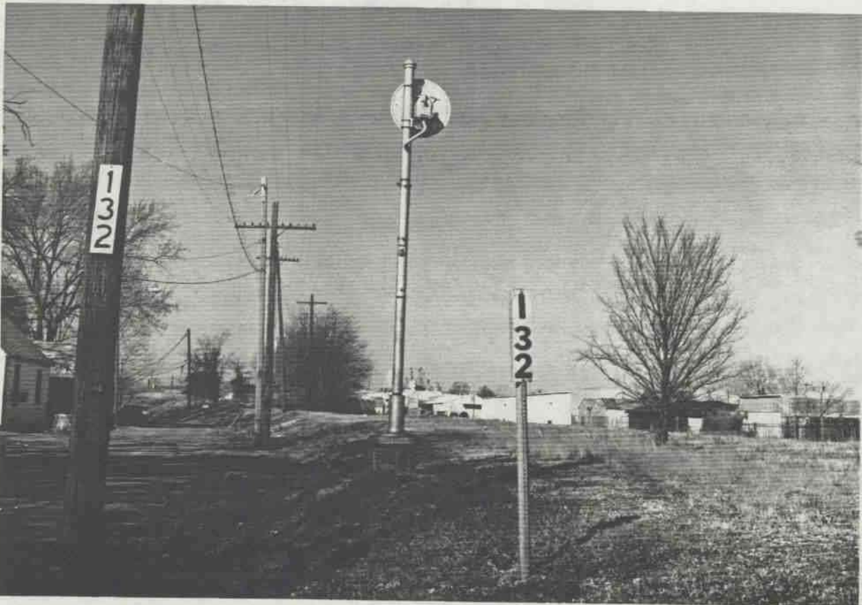
At Rock Island Main Line Southern Division milepost No. 132 (North Little Rock) the one-lens, three color signal for eastbound (to Memphis) trains is now a lifeless eye staring into space, where trains have rolled into history. (Gene Hull, March 1991)
