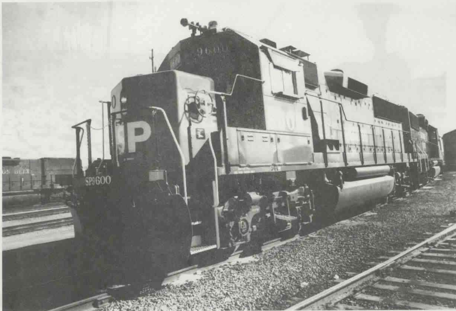
New Southern Pacific GP60 at Kansas City March 1988. This is the first one off the line of the 20 being built by EMD (numbered 9600-9619). These units have 3800 horsepower. SP has also ordered 40 GE diesels (B40-8, 4,000 HP units numbered 8000-8039). All these new engines are state-of-the-art units with computerized components for easier trouble-shooting and fuel efficiency. (Jim Johnson photo, Cotton Belt Public Relations)
