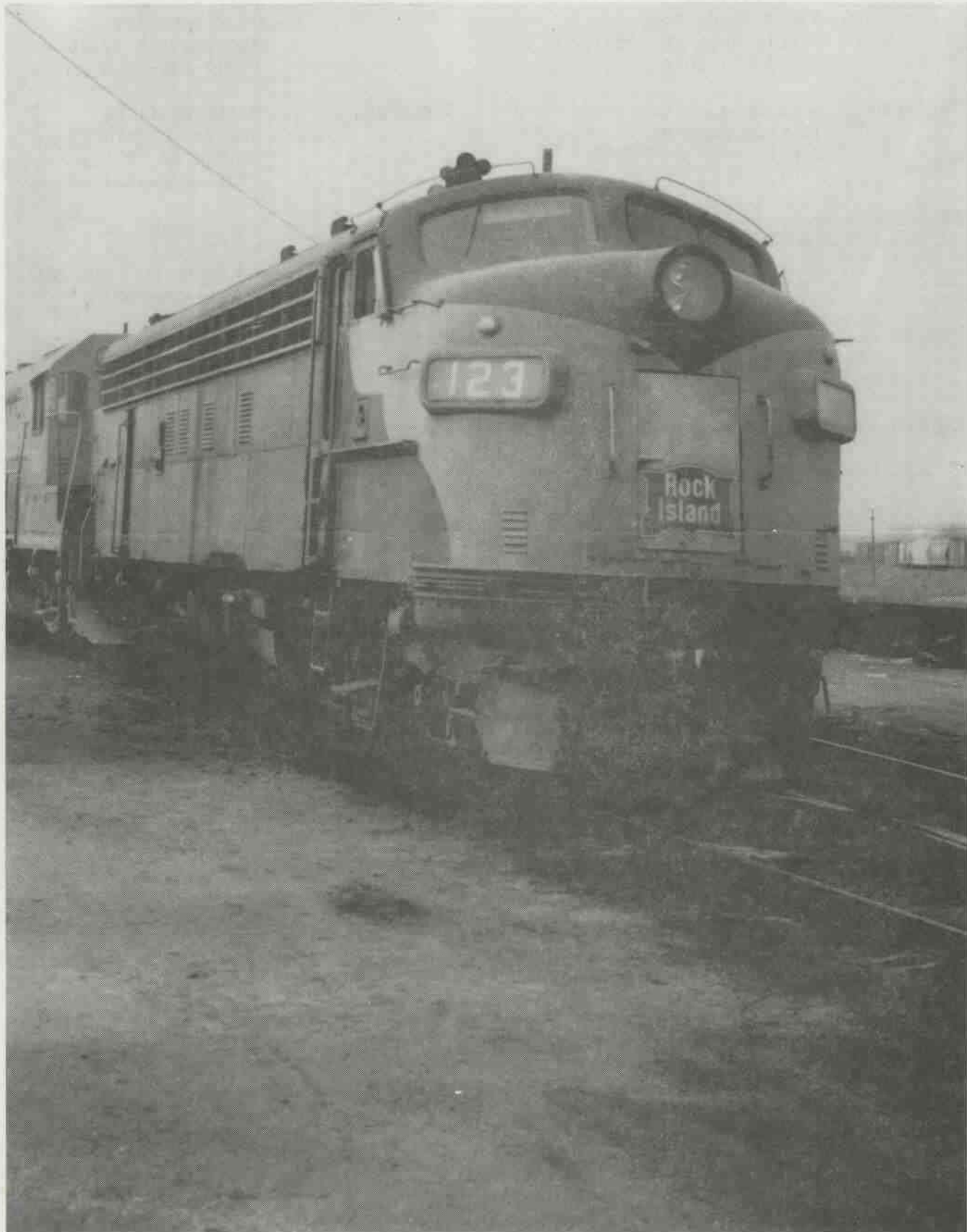
ROCK ISLAND EMD F7 #123 at Little Rock, Arkansas on February 24, 1975. It was built in 1951 with 1500 HP, max speed 71 MPH and gear ratio 61/16. This was the same type of engine used in L.T. Walker's story on Rock Island Train #991 (which derailed while westbound between Little Rock and Booneville in 1949). Mr. Walker's story begins on page 3. (Photo by Bill B. Bailey)
