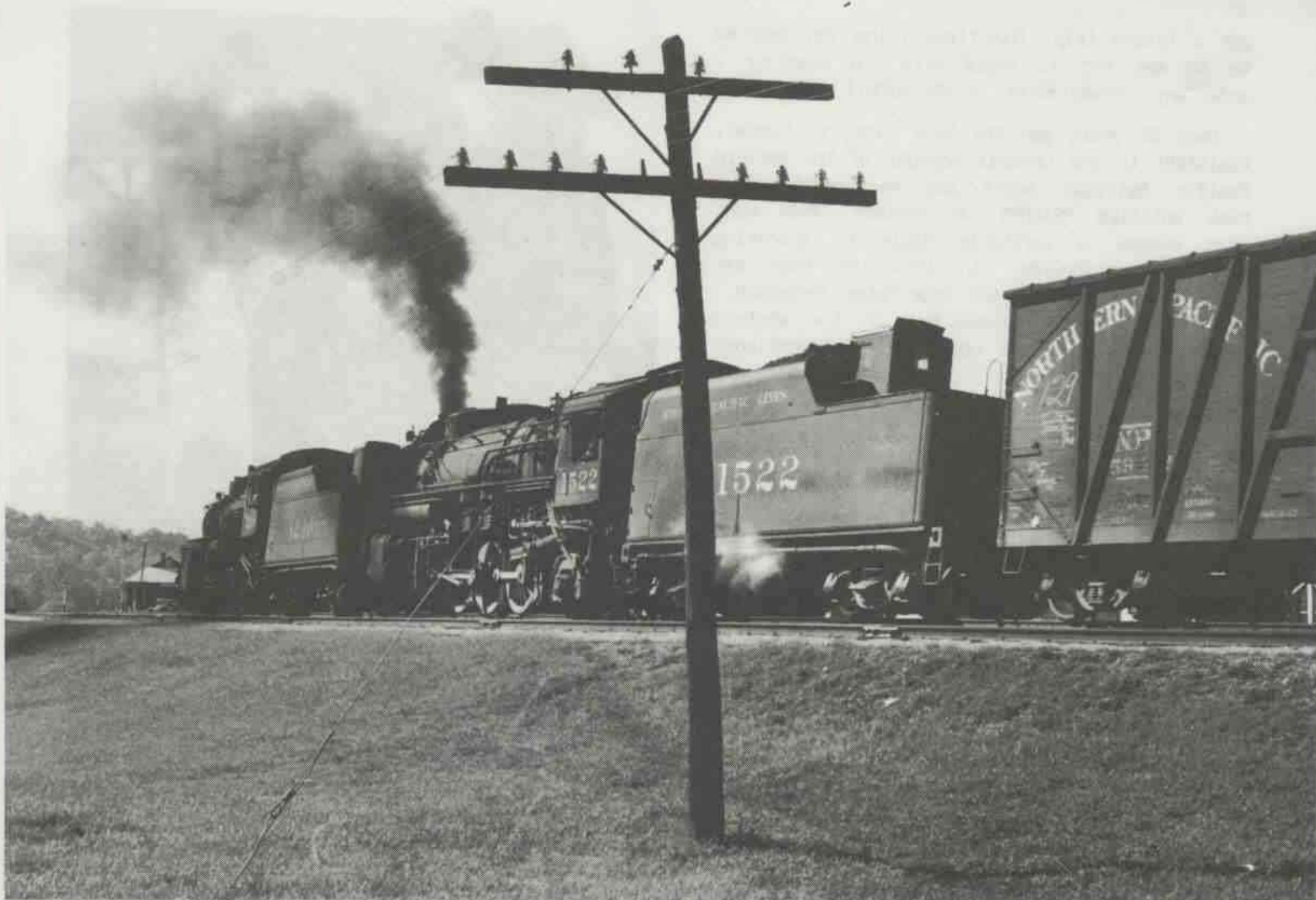
Missouri Pacific Train 261 approaching station at Branson, Missouri on the old White River Division. Train order signal in STOP position for this train indicating orders on hand. Engine 1522, a heavy booster-equipped 2-8-2, is road engine with 1230, light 2-8-2 as helper. This is the foot of the hill and White River is to the left. Soon after leaving station they hit a ten mile 1% pull to the Arkansas state line near Crest Tunnel. Late 1940s. (J.G. Collias collection)
