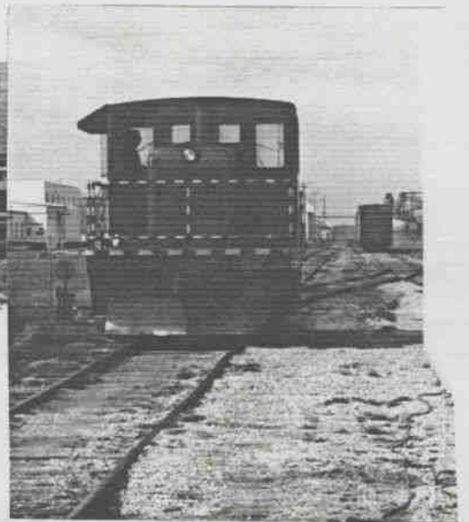
DVS engine number 50 300 hp GE switch engine built 5-54.
