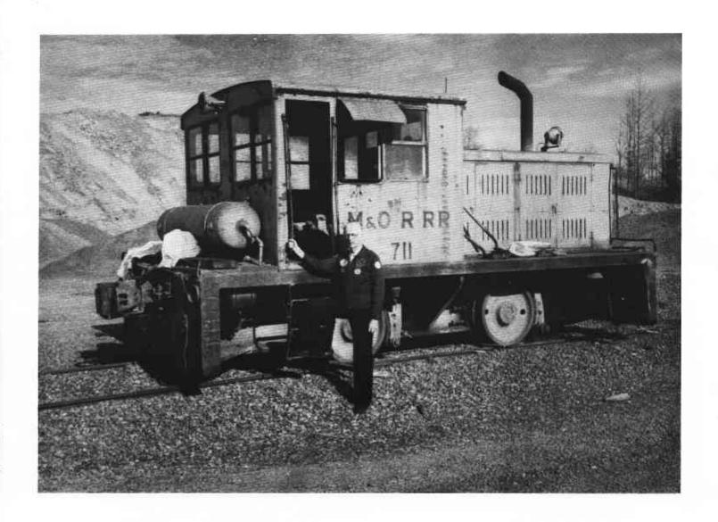
A lonesome little locomotive that resided in a gravel pit near Malvern, Arkansas in 1989. According to J. Cary Nettles of Hot Springs, this engine appears to be unique in that it apparently started out to be a Caterpiller bulldozer but somewhere the genes got mixed up. Note the outriger air compressor. Mr. Nettles thinks the M&O RR stands for the Malvern & Ouachita River Railroad. Is he right? (J. Cary Nettles photo)
