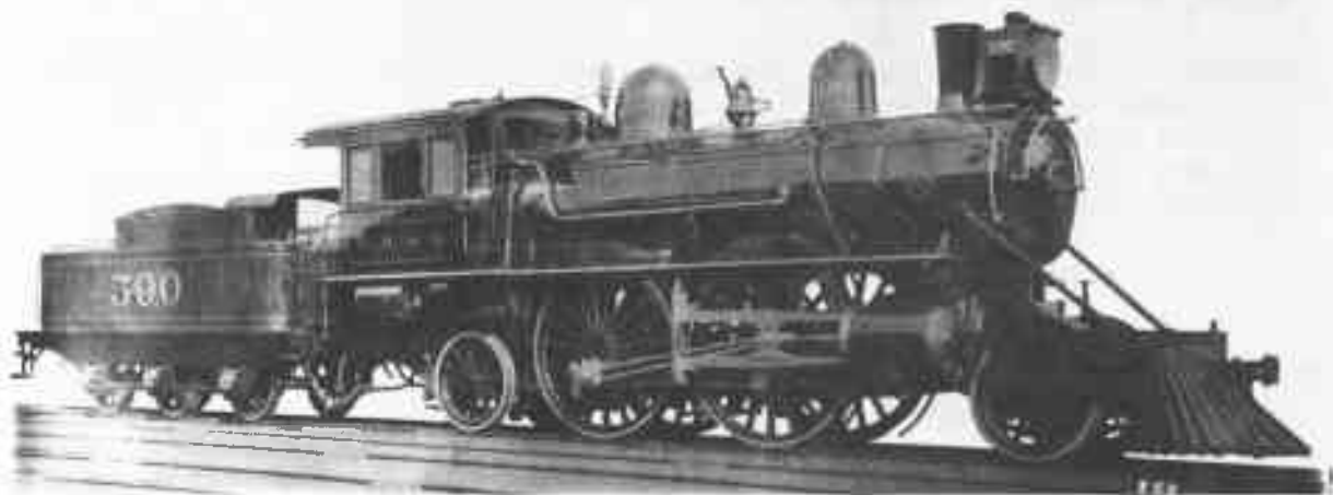
First wide bituminous burner - CB&Q 2-4-2 No. 590, by BLW 1895. (Gene Hull collection)
