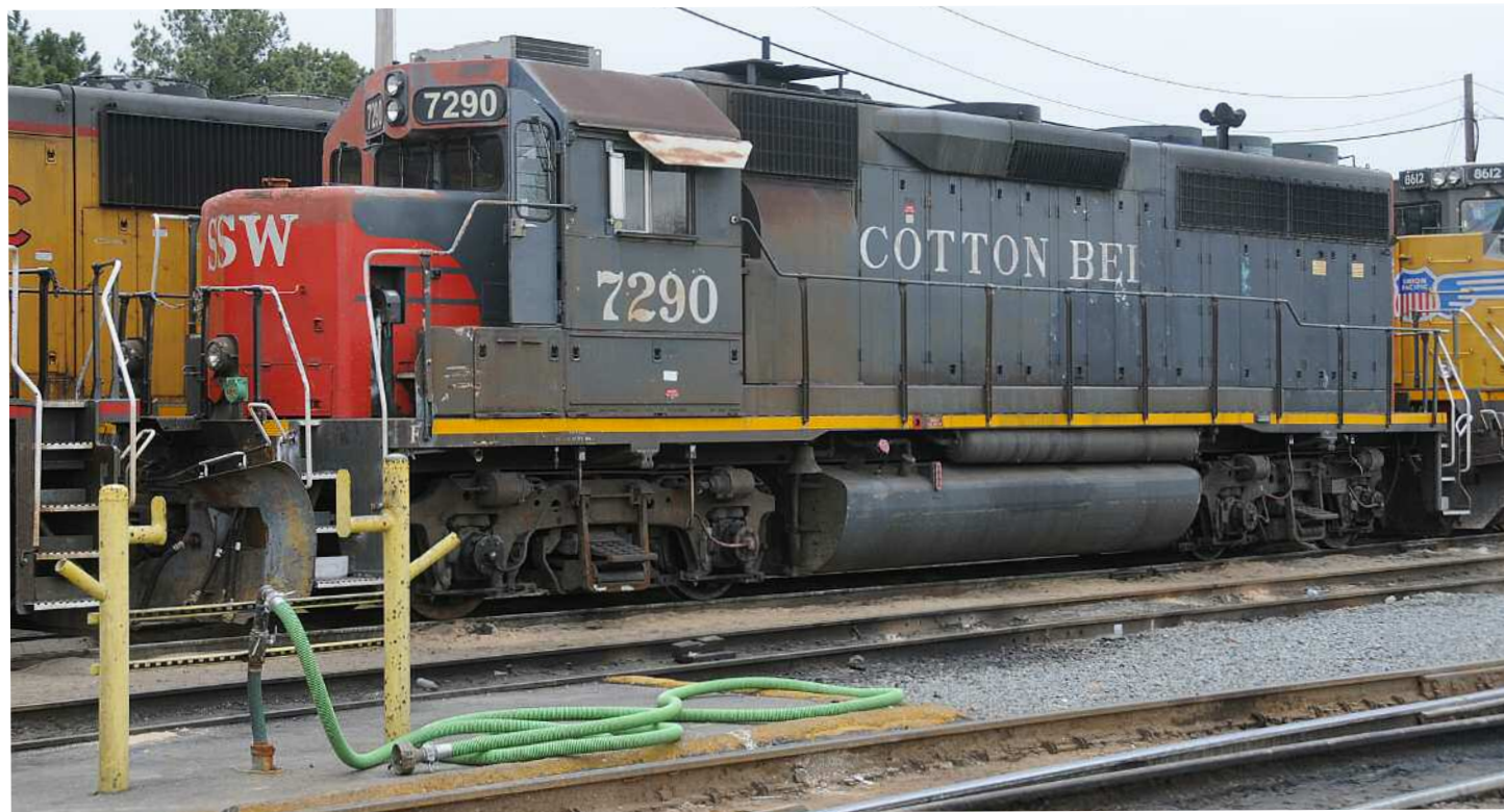
St. Louis Southwestern No. 7290, a GP40M-2 was spotted at Union Pacific's service ramp in North Little Rock, Arkansas, on February 14, 2010. The unit was built in May 1970 and rebuilt in January 1991. The unit is basically unaltered except for the FRA mandated yellow-frame stripe. Photo by John C. Jones.
